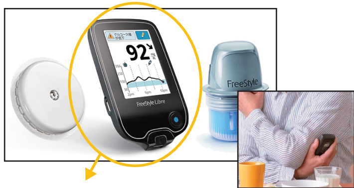
FGM (Flash glucose monitoring) /isCGM (Intermittently scanned CGM) = 間歇スキャン式持続血糖モニター
